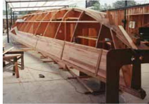
All bulkheads are foam filled, plywood sided and finished with varnished epoxy coated tongue and groove cedar veneer.
